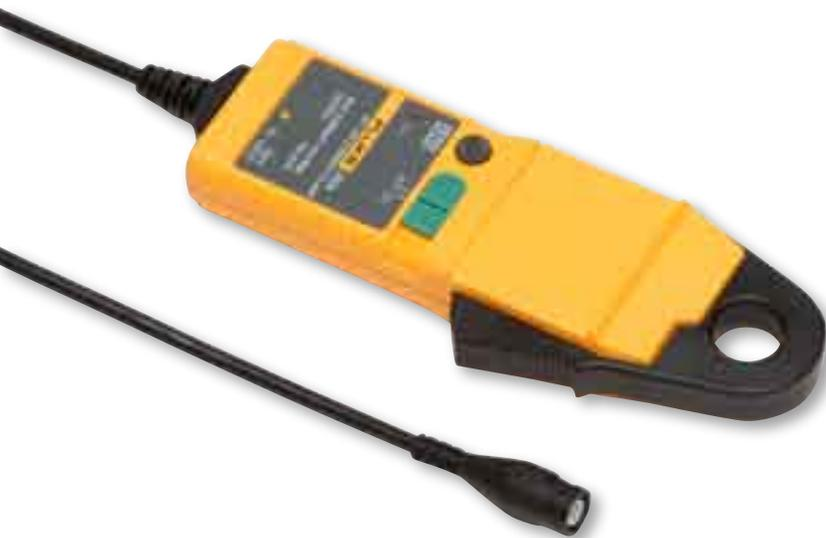
The i30s current clamp is based on Hall effect technology for use in measurement of both dc and ac current. The i30s may be used in conjunction with oscilloscopes and other suitable recording instruments for accurate non-intrusive current measurement.
