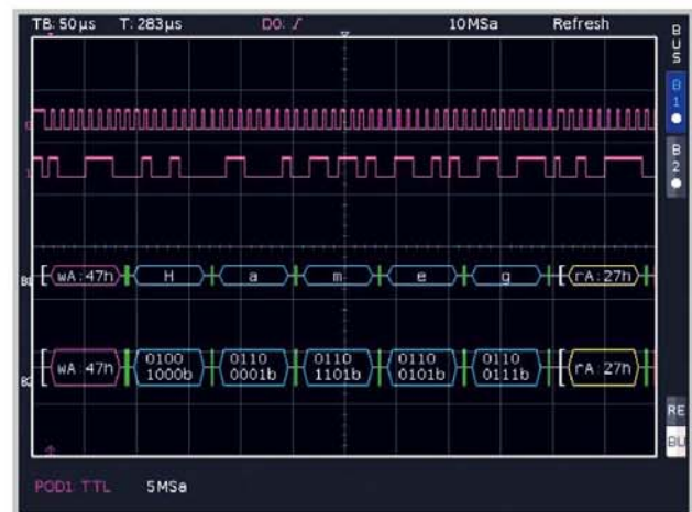
I 2 C Bus ASCII and Binary Decode of the Digital Channels
