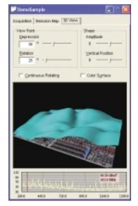
With the "3D View" function, a field intensity distribution is represented graphically. The higher the intensity, the higher the altitude. This 3D graphic rotates for easier identification.
