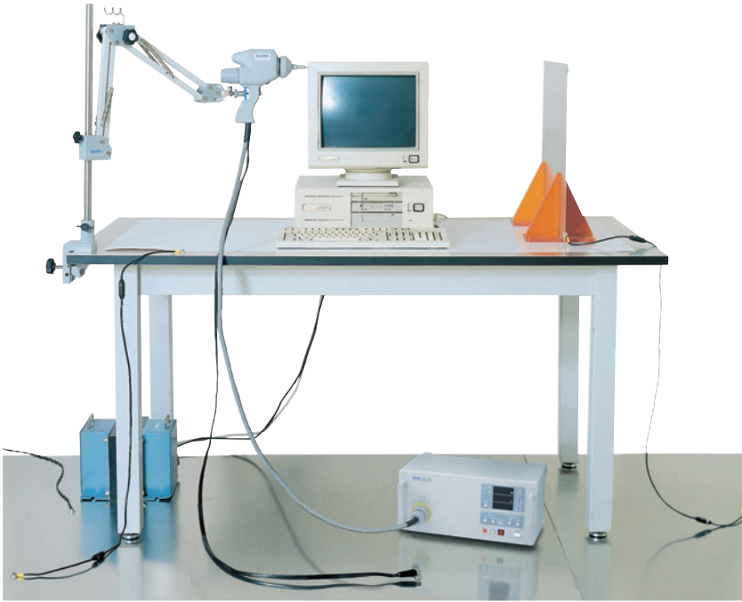
Test set-up example with ESS-801
