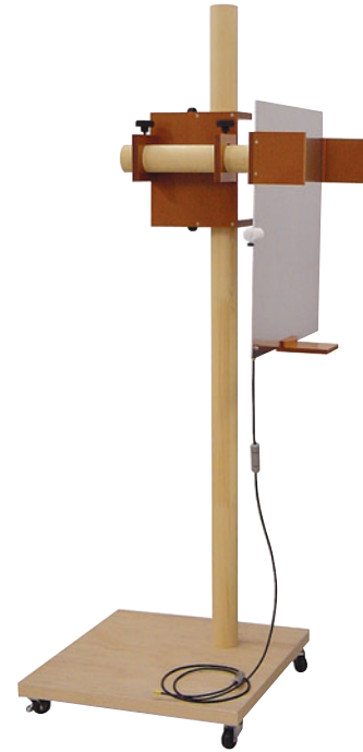
ESS-801GL (Vertical coupling plane & Cable with resistors)
